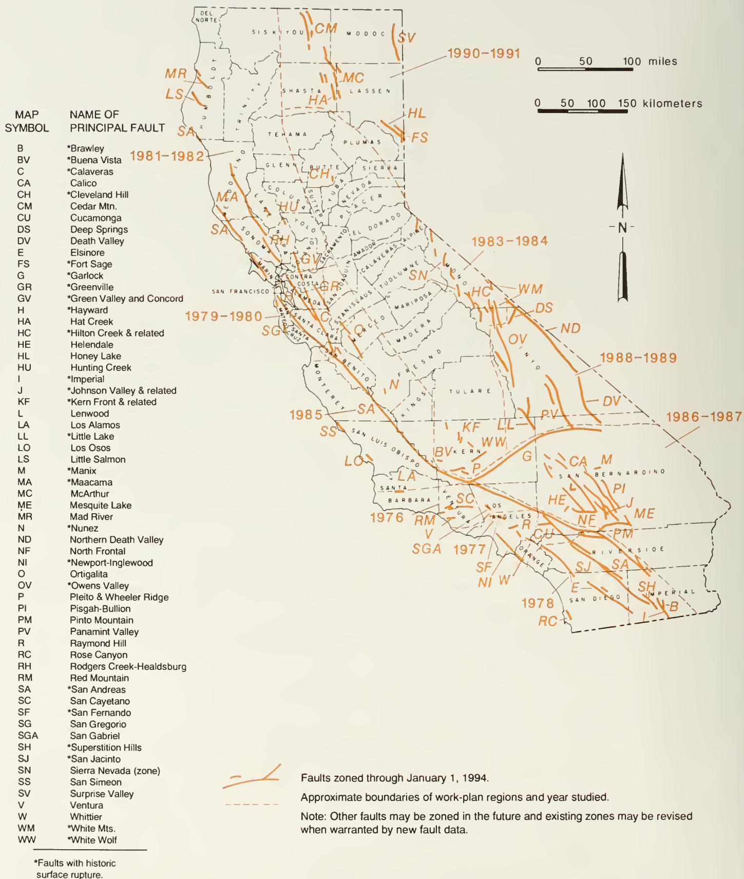
Figure 1. Principal active faults in California zoned under the Alquist-Priolo Earthquake Fault Zoning Act. Dashed lines and dates identify recently completed work-plan for 10 regions and when studied.
